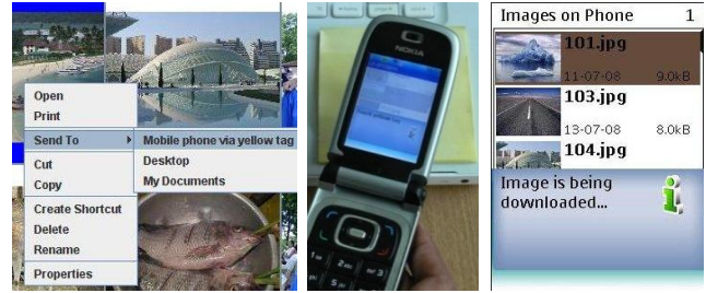
Figure 7. Downloading a picture from the phone to the laptop with touch & connect
