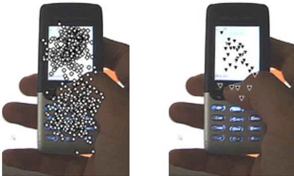
**Figure 4: Eye gaze positions during a task, overlaid over the phone in use. Left: write a text message. Right: set alarm time.**
