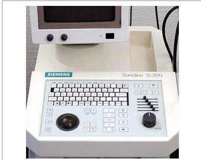
Figure 2. User interface of an ultrasound system with a standard keyboard, knobs, sliders, buttons and a trackball.
