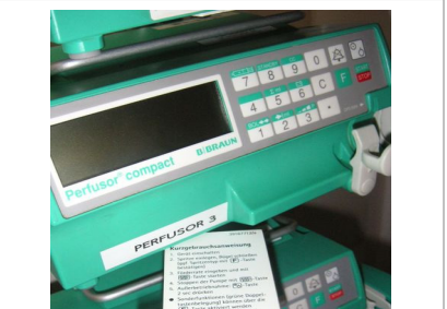
Figure 3. User interface of a professional proportioning pump with a plastic foil keyboard.
