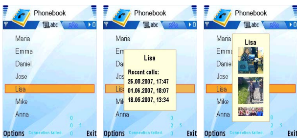
Figure 3: Phonebook application with two types of pop-up info screens that appear when touching the select key.
