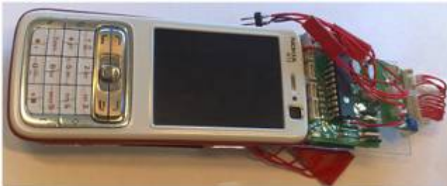
Figure 1: Nokia N73 with Microcontroller + Bluetooth board and AD7142 touch sensor board (far right) attached to the top.
