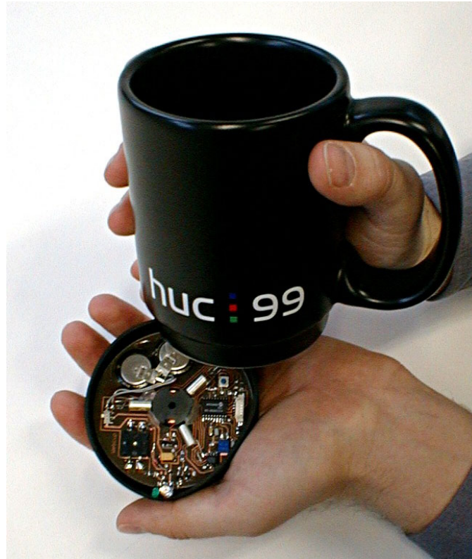
Fig. 9 The MediaCup, a device for implicit interaction (Beigl, Gellersen, and Schmidt, 2001)
