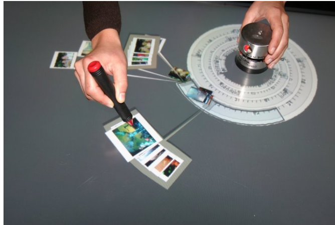
Fig. 12 The Photohelix: A hybrid physical-digital interface (Hilliges, Baur, and Butz, 2007a)
