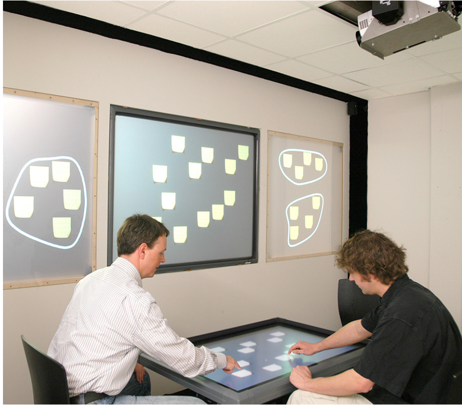
Figure 6: Overview of our room with the wall-sized display in the background, the steerable projector on the ceiling, and an interactive table in the foreground.
