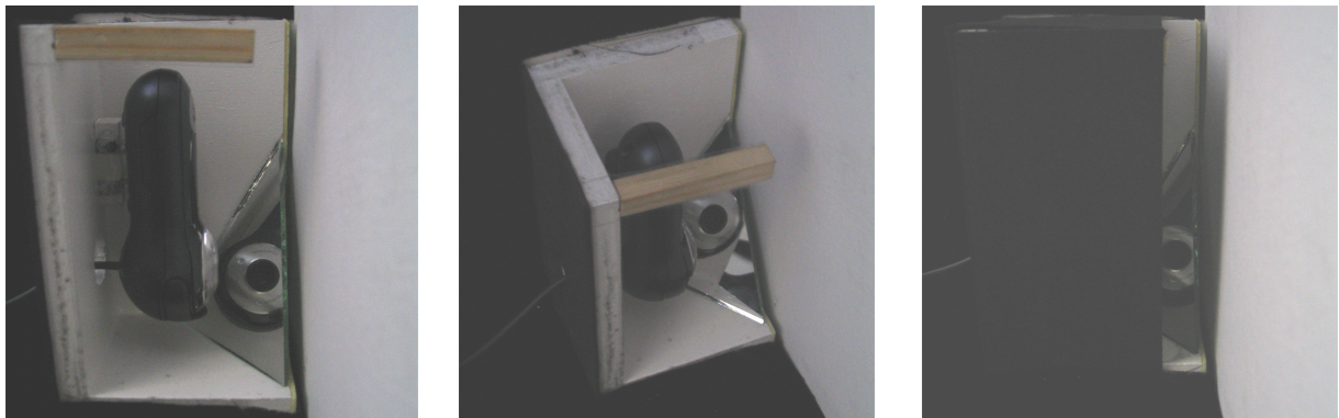
Figure 2: Different views of the fixation for one camera. Left and center show the fixation without the black foamed rubber on it. Right shows the final fixation attached to the wall.
