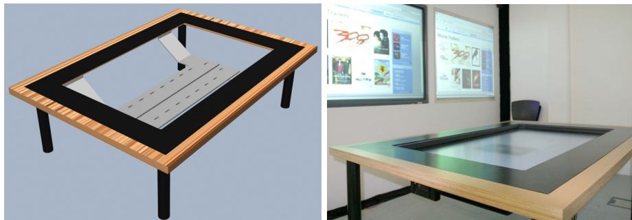
Fig. 1. Left: Construction drawing of our interactive table frame, built to hold a 42 inch LCD screen with a DViT overlay panel. Right: The actual table, integrated in our interactive environment
