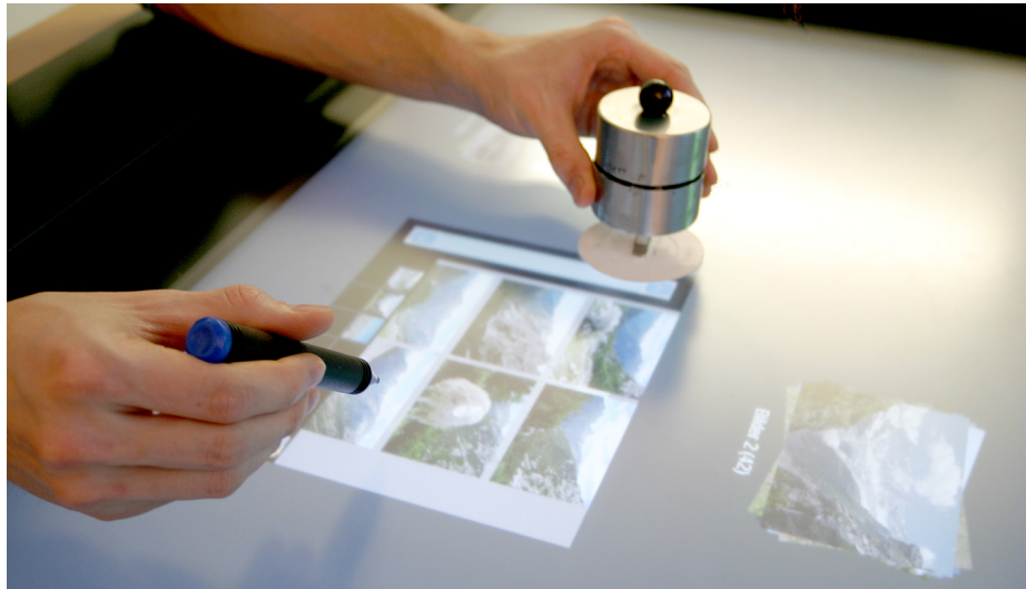
Fig. 4. PhotoLens in use on our interactive Tabletop: The non-dominant hand holds the physical handle of the lens and moves it over piles of photos. Turning the handle zooms in and out of the pile's content, sliding the handle along the side scrolls through the content. The dominant hand uses a pen or a finger to select and move photos.
